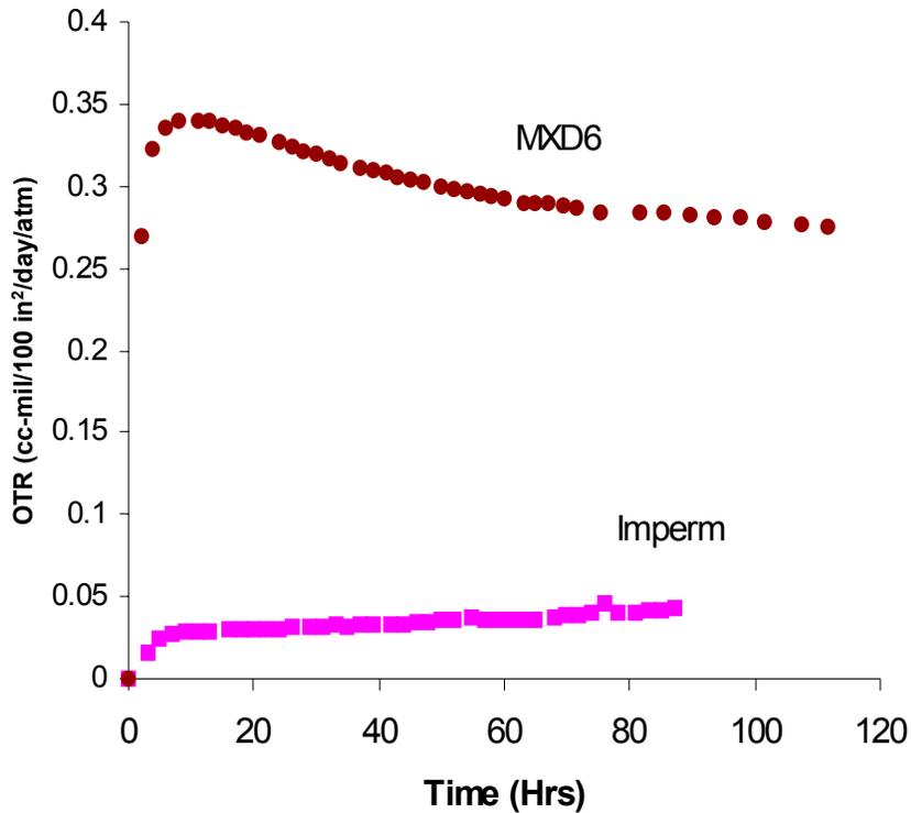
A 16 ounce, tri-layer blow molded non-pasteurized beer bottle illustrates the benefits of Imperm. This package contains a 10% barrier layer, sandwiched between PET. Because Imperm's process window overlaps that of PET, typical preform injection and blow molding process conditions are used. Since Imperm's matrix is nylon, it exhibits good adhesion to PET without the need for tie-layers.
